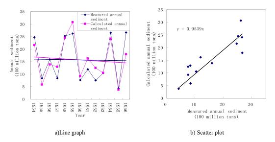
Fig. 5 Comparison of measured annual sediment transport volume with calculated annual sediment transport volume in 1954-1966 period
