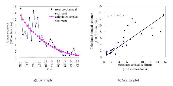
Figure 8 Comparison of measured annual sediment transport volume and calculated annual sediment transport volume from 1988 to 2015 period
