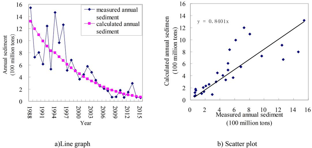
**Figure 8 Comparison of measured annual sediment transport volume and calculated annual sediment transport volume from 1988 to 2015 period**
