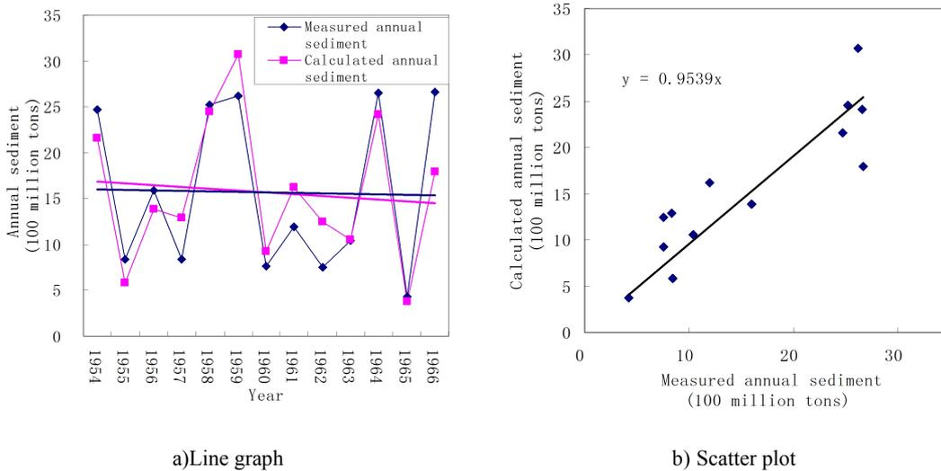
**Fig. 5 Comparison of measured annual sediment transport volume with calculated annual sediment transport volume in 1954-1966 period**
